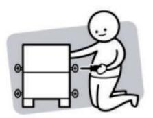
Do not fully tighten all screws until step/ precess finished.
